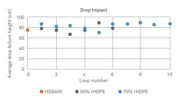
Figure 8. Top Load and Drop Impact, two important bottle properties, were maintained throughout the loops
