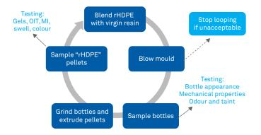
Figure 4. Laboratory model schematic. Regrind was also used during at each loop to emulate the commercial scale process.
