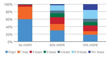
**Figure 3.** Steady state heat exposure for different PCR levels, assuming 40% regrind (primary recycling). One loop defined as the equivalent of modelled recycling extrusion process.
