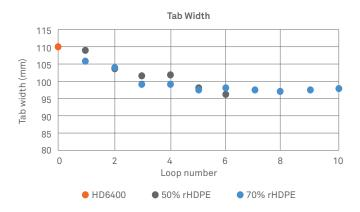
Figure 5. Tab width as a function of thermal processing
