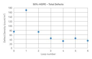
Figure 6. Defect levels measured (50% rHDPE)
